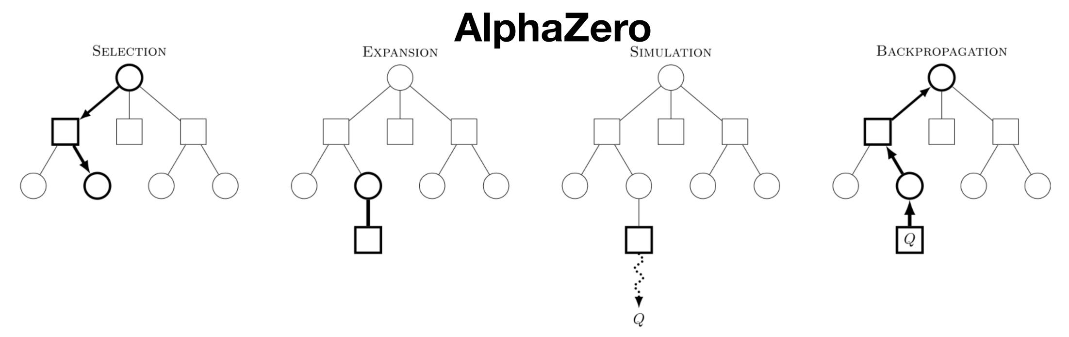
**Obtaining the** *t***-th rollout** (steps called **Selection/Expansion/Simulation)**:
