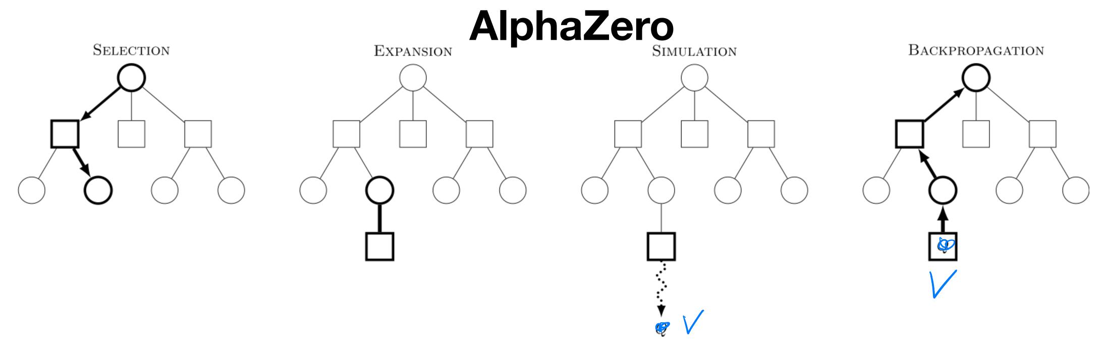
**Obtaining the** *t***-th rollout** (steps called **Selection/Expansion/Simulation)**:
