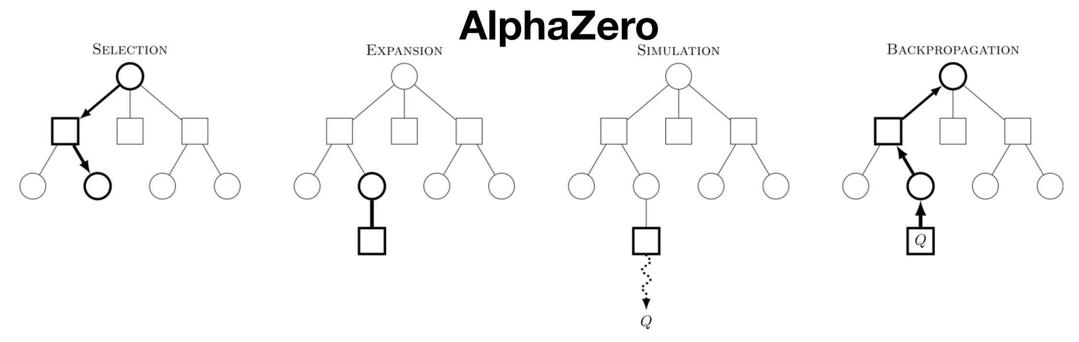
Obtaining the *t*-th rollout (steps called Selection/Expansion/Simulation):
